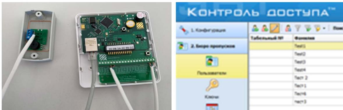
Figure 2: Hardware and software part of the ERA 500 network controller.
