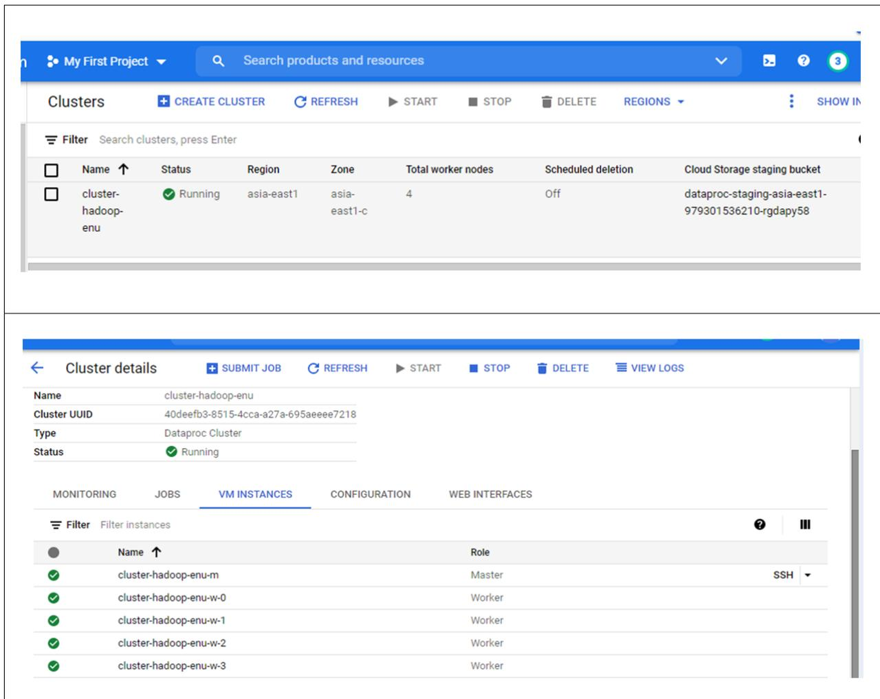
Figure 5: The process of configuring the Hadoop cluster via GCP.
